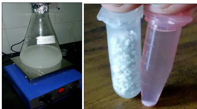
Fig 1: Chemical synthesis of zinc oxide nanoparticles
